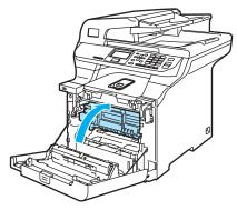
When you replace the belt unit with a new one, you need to reset the belt unit counter by completing the following steps:
